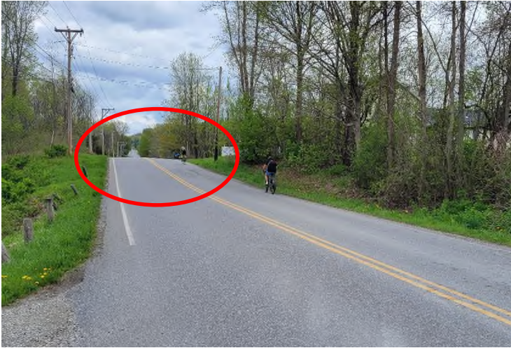
Figure 4: Difference in vertical elevation creating a crest, looking towards east
